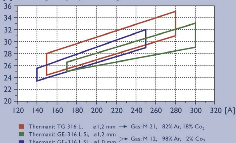
[V] Welding in Spray Arc Range
