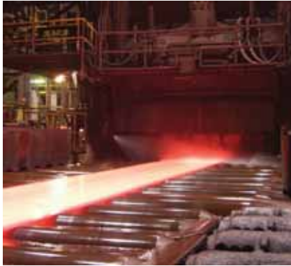
1. Rolling of base and clad material
